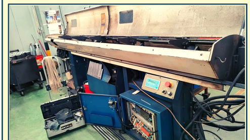
Repair Barfeeder LNS
